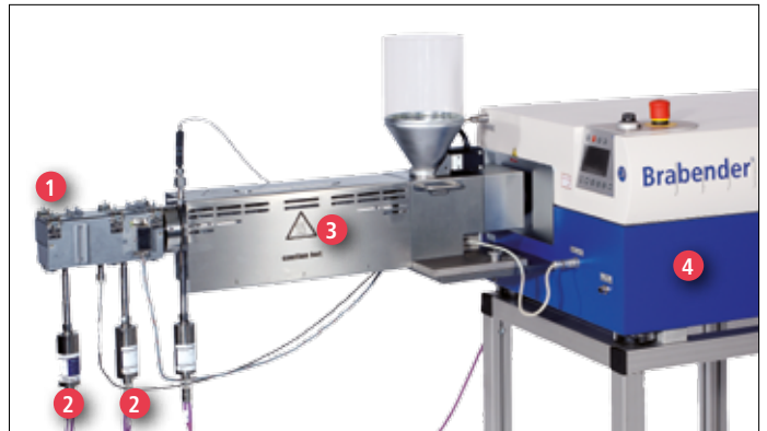
Extruder 19/25 with slot capillary die head
